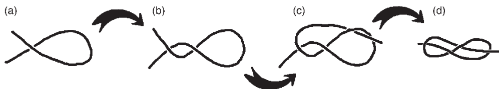
Figure 4. Figure-of-eight or Flemish knot. The rhyme to forming the knot is ‘Twist it once, twist it twice; pass it through and make it nice’ [28].
